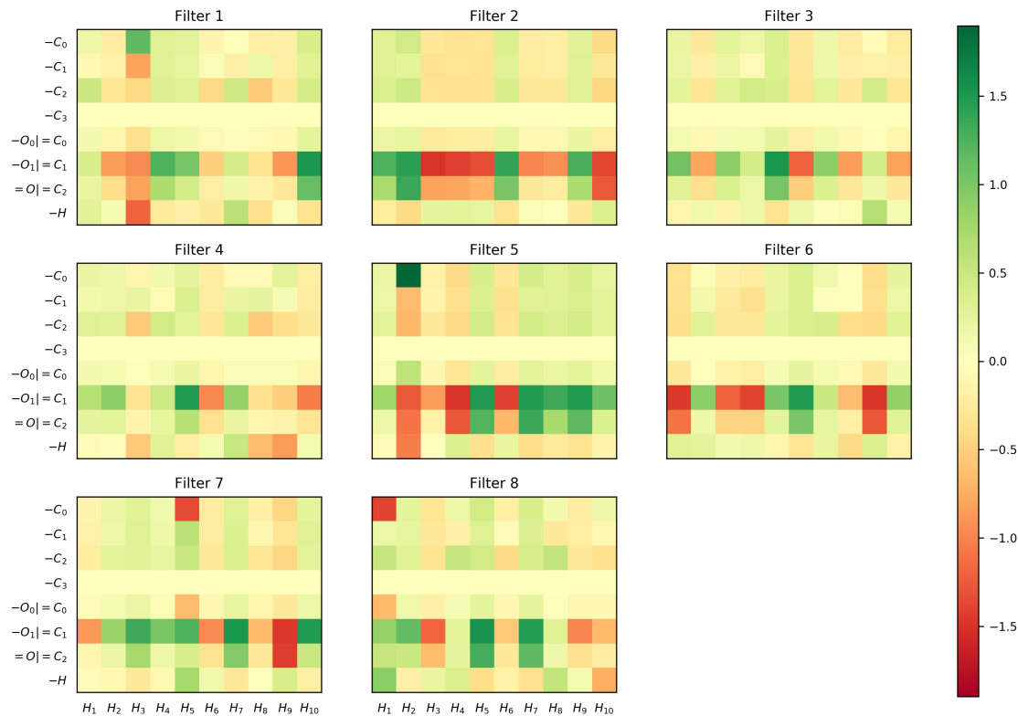
Figure 3.7: Weight matrices for the 8 filters learned by running our proposed model. Each of the eight 8-by-10 matrices contains the values of the weights that connect each of the 8 atomic fingerprint values (which, according to Figure 3.4 are the number of different bond types an atom is connected to) to the 10 hidden units denoted as H_1 to H_{10} (the left half of each subnetwork or filter shown in Figure 3.5).
